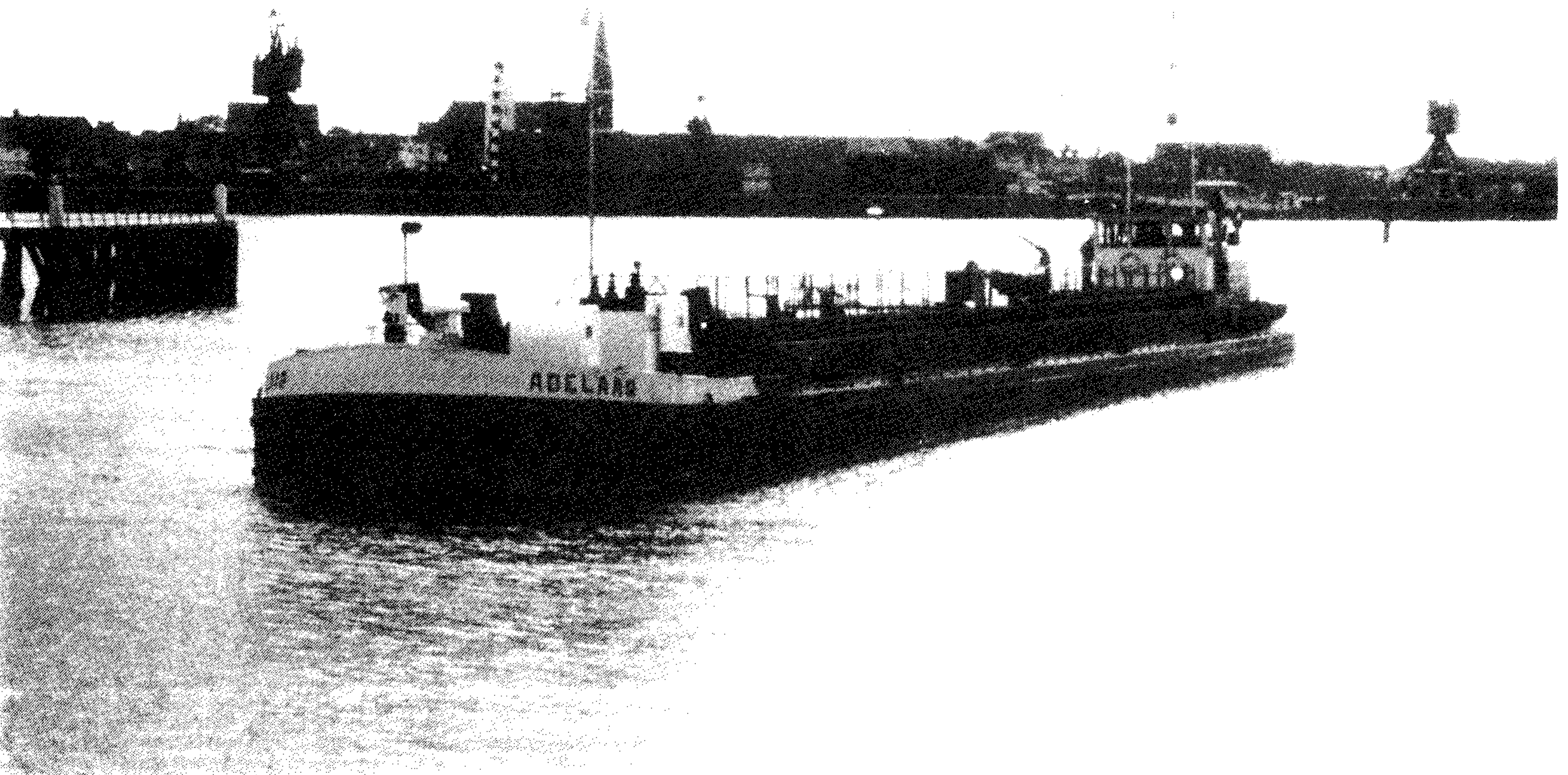
Figure 5e. The "Adelaar" a small trailing suction hopper dredger owned by Dutch Dredging.
