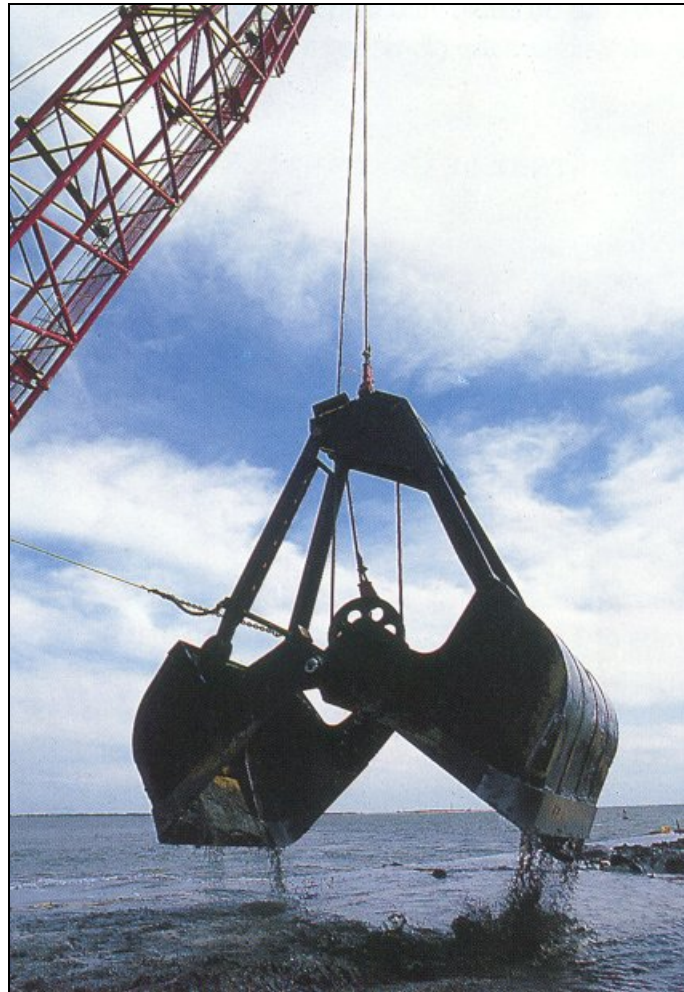
Figure 18: The 50 cubic yard clamshell buckets.
